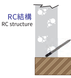
◎ 二次層縫止漏 2 leaking sealing works of layer cracks
