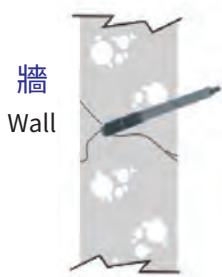
◎ 裂縫止漏 sealing works of construction cracks
