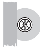
落水管四周 加強一度防水 First waterproof around rainspout
