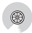
以落水管為中心 塗佈一底一度防水 Take rainspout as the center to do spreading and laying waterproof works
