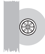
落水管四周 加強一度防水 First waterproof around rainspout
