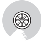
以落水管為中心 塗佈一底一度防水 Take rainspout as the center to do spreading and laying waterproof works
