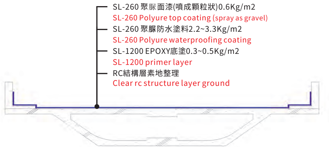
SL-260-橋樑面防水防蝕示意圖 SL-260-1 bridge face waterproof and corrosion proof sketch map
